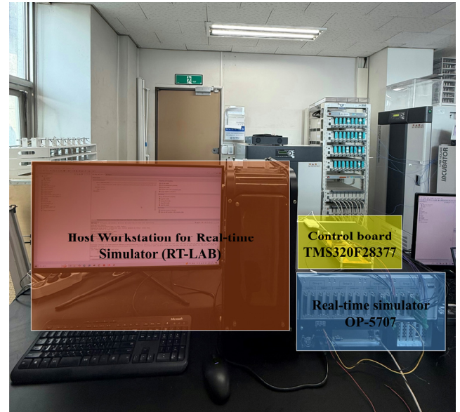
FIGURE 13. HILS-based experimental setup for validating the proposed EKF-LQR-based current controller.
