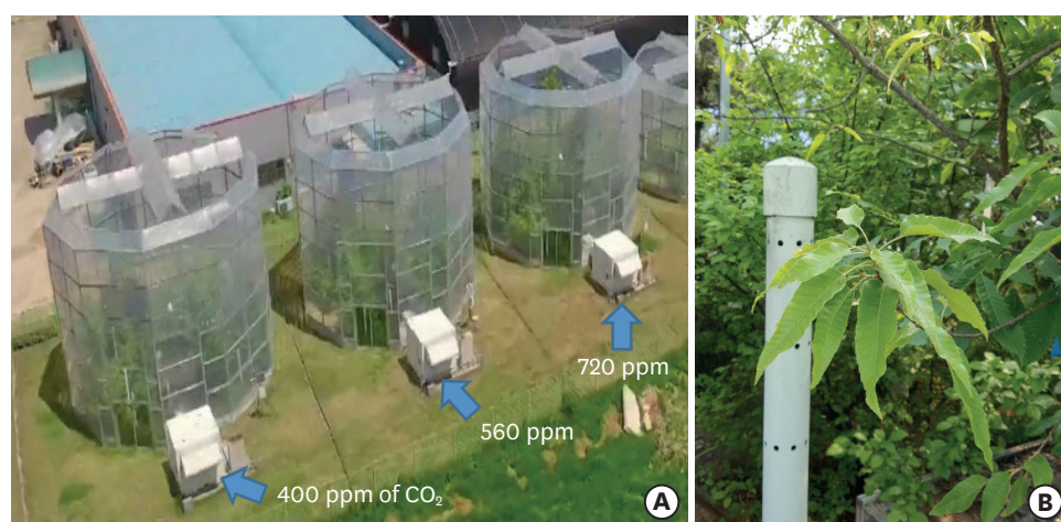
Fig. 1. (A) Open top chambers at the National Institute of Forest Science in Suwon, Korea. (B) Internal view showing a CO 2 injection nozzle and plants. Permitted from Kim KR, Oh JW, Woo SY, Seo YA, Choi YJ, Kim HS, et al. Int J Biometeorol 2018;62:1587-94. 20
