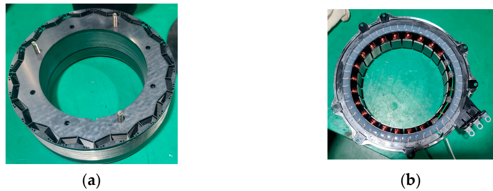
Figure 23. Final model production photograph: (a) Rotor production model, (b) Stator production model.
