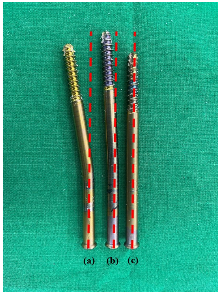
Figure 7. Photographs of the reconstruction screws in groups 1 and 2 after the lateral impact test. Single reconstruction screw (a) in group 1, lower reconstruction screw (b) in group 2, and upper reconstruction screw (c) in group 2. The red dashed lines represent the straight longitudinal axis drawn through the distal part of each screw body, serving as a reference to visually highlight the degree of bending. Note that the screws are bent in the following order: single reconstruction screw in group 1, lower reconstruction screw in group 2, and upper reconstruction screw in group 2.
