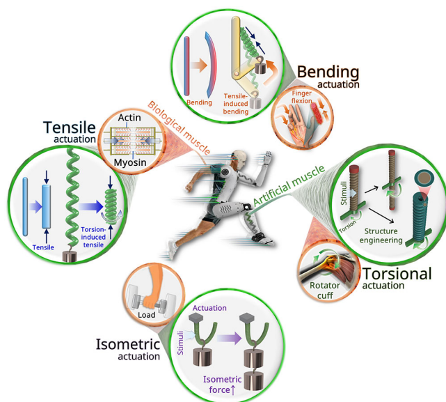
Fig. 1 | Overview of actuation in fiber-type artificial muscles for robotics and biological muscles, categorized into tensile, bending, torsional, and isometric actuation.
