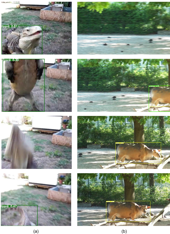
FIGURE 5. We show two failure cases. Boxes are the predictions of DiffusionVID with ResNet-101 backbone. In case (a), the 'lizard' is moving quickly, causing severe motion blur. Our method fails to detect the lizard in third frame. Case (b) shows the partial occlusion of a 'cattle' as the camera moves. Our method misclassify hind legs of a 'cattle' to 'antelope' in second frame, and recovers at following frames.
